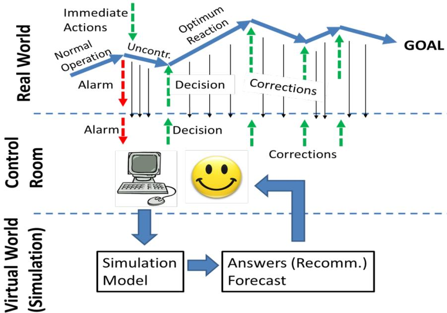
Figure 3: Principle of Real Time Physical Simulation for Emergency Management.
