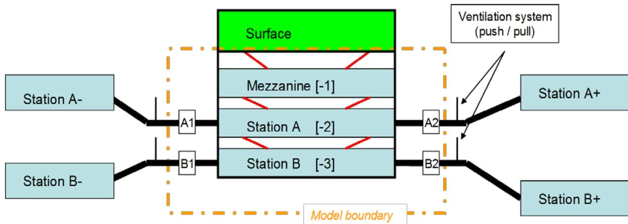
Figure 1: Physical representation of a generic metro station.
