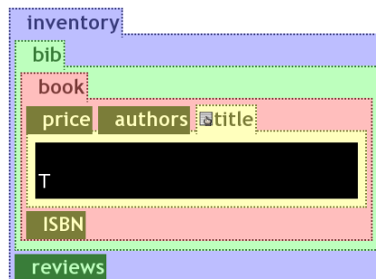
Fig. 6. Example with folded content (the tabs labelled "reviews", "price", "authors" and "ISBN") and context menu button (at the tab labelled "title")
