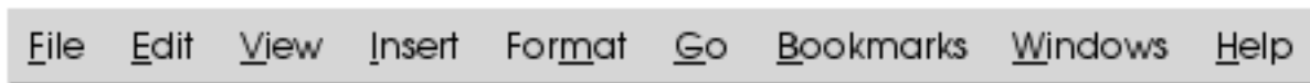
Figure 4.9. A menubar showing all the standard menu titles in their correct order
