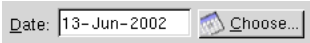
Figure 6.5. Text entry field requiring a date as input, with a button beside it to pop up a GtkCalendar control to simplify the task
